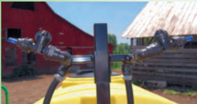
Hypro Boom X Tender with Diaphragm Check Valve/Nozzle Body
